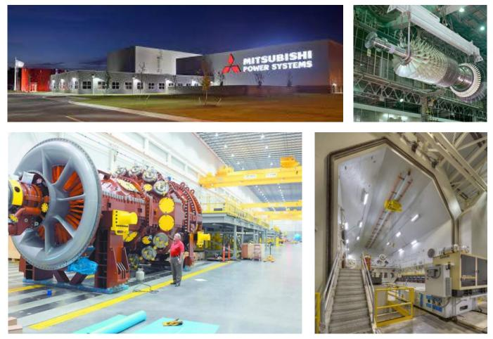
Bennett & Pless Structural B&P provided the structural design of the 440,000 SF facility including a 381,000 SF manufacturing/ refurbish turbine parts building, a 20,000 SF bunker/ turbine balancing facility with a 61,000 cubic foot vacuum chamber, a 17,000 SF conference center and a 10,000 SF maintenance building. The manufacturing buildings were designed with 60-90 foot clear span heights for overhead heavy bridge cranes and hook heights that reach up to 60 feet.
