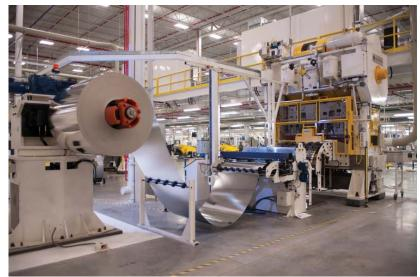
The renovation of an existing 530,000 SF building on an industrial site included improvements for use as a food-grade steel can stamping, manufacturing and warehouse operation.
